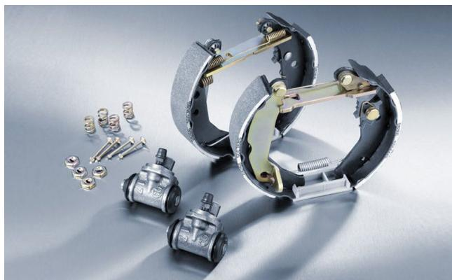
The brake shoes are also the carrier of the friction material. During braking, there is natural wear of the friction material. The decreasing thickness of the friction material is compensated by a mechanical adjustment mechanism. However, it can only be compensated if there is sufficient friction material. When the wear limit is reached, the entire brake shoe must be replaced.
