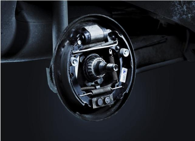
The wheel cylinder is a safety-relevant vehicle part. It should be checked regularly as part of regular service and maintenance to ensure that it is perfect working order. When the brake shoes or the brake drums are replaced, it is advisable to replace the wheel cylinder at the same time. This will avoid follow-up repairs having to be made soon after.
