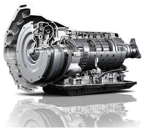
Instead of a separating clutch, automatic gearboxes are provided with a so-called hydrodynamic torque converter for starting. The engine does not have to be disconnected from the gearbox, as automatic gearboxes are shifted under load and thus transmit the engine torque even during gear change.
