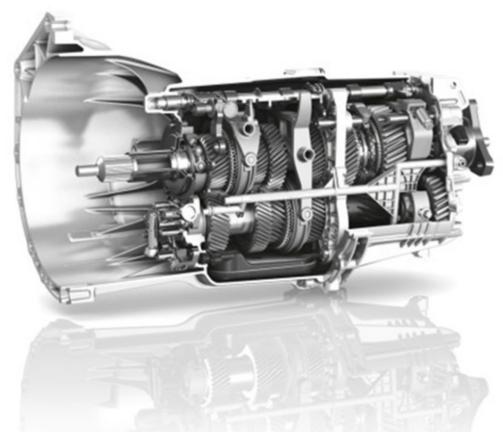
In manual gearboxes the speed of the engine is introduced by way of the input shaft. The output speed, i.e. the speed leaving the gearbox, is the product of various transmission ratios arising from the different speeds of the meshed gears.
