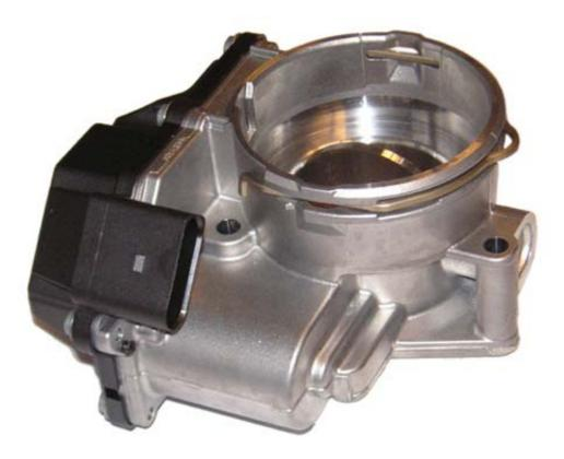
If throttle valves are used in diesel engines, they are generally referred to as air management valves. Air management valves can be with or without integrated control electronics. As indicated above, air management valves throttle the intake air in the intake air system of diesel engines via electromotive means in order to achieve precision controlled exhaust gas recirculation and prevent the inconvenient shaking that would otherwise occur when the engine is switched off.
