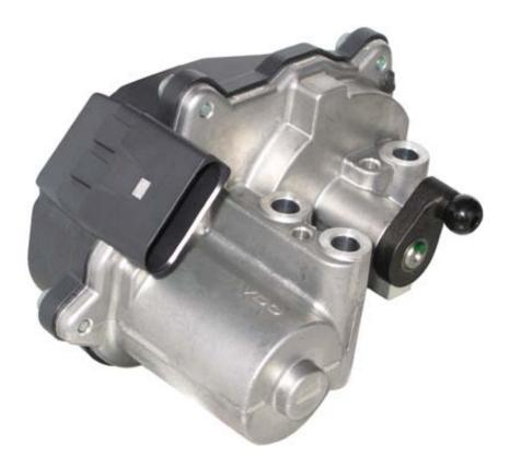
Air flap servomotors are electrical actuators with integrated position sensor and optional integrated electronics. They facilitate the continuous adjustment of intake pipe flaps or turbocharger guide vanes, for example, and, by means of more precise control, are able to replace conventional pneumatic drives which are no longer sufficient for the advanced requirements that have to be met.
