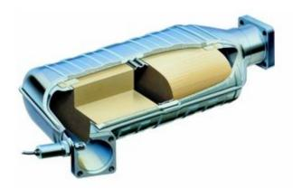
A catalytic converter consists of a stainless steel housing that contains either a metallic (metalith) or ceramic (monolith) substrate. This substrate features numerous small longitudinal channels, designed to maximise the surface area for optimal efficiency. The surface of the substrate is coated with a highly porous wash coat layer, into which precious metals, such as platinum, palladium, and/or rhodium are embedded.
