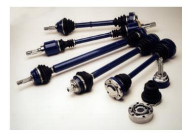
Drive shafts for cars with front wheel drive consist of the outboard fixed joint, the inboard constant velocity joint and the connecting shaft. They also include elements such as the anti-lock system ring and the torsion damper. The basic design of the outboard fixed ball joint, the constant velocity joint, dates from the 1930s.
