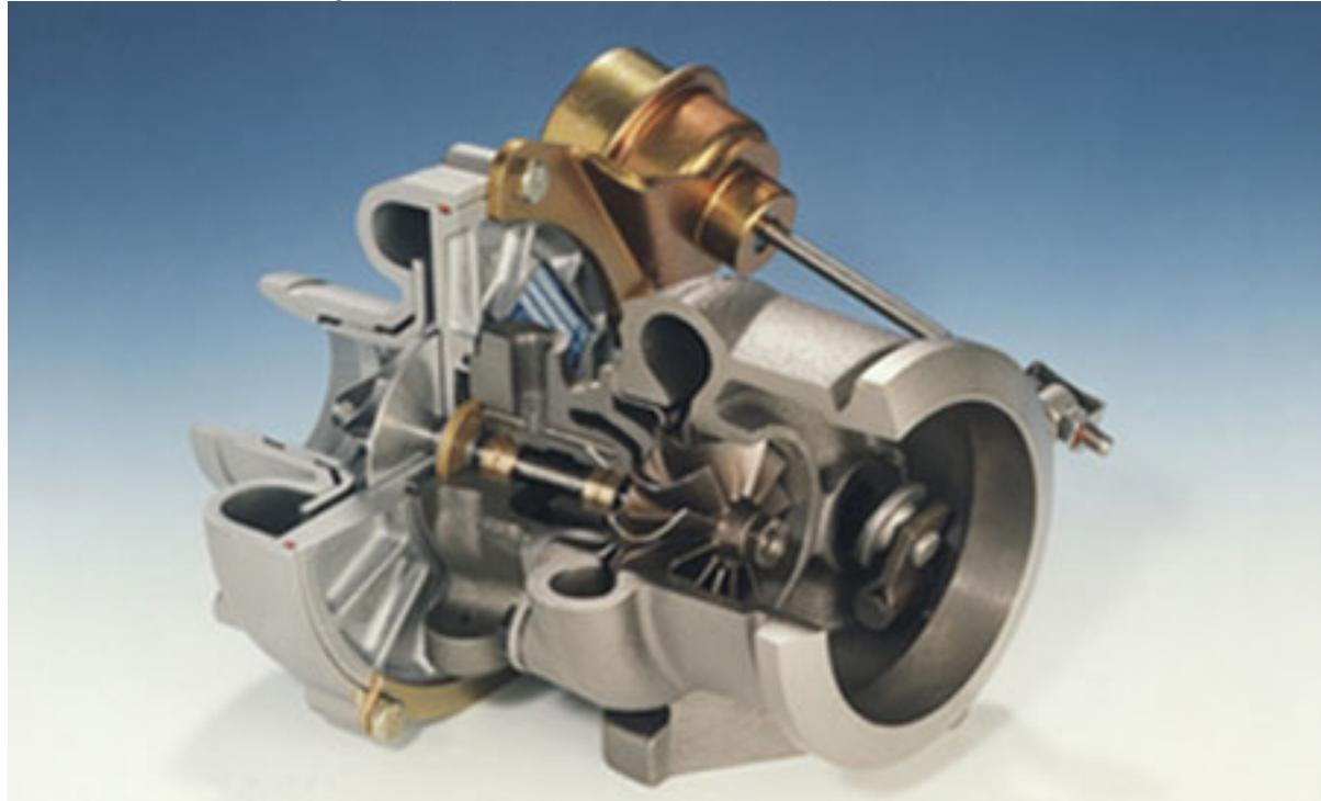
a fixed mechanical connection established via a common shaft. The turbine is driven by the exhaust gases from the engine and supplies the drive energy for the compressor. In most cases, centripetal turbines and centrifugal compressors are used for turbochargers.
