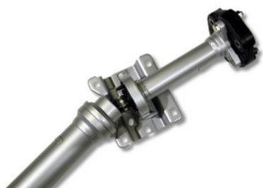
The longitudinal shaft or cardan shaft is a
