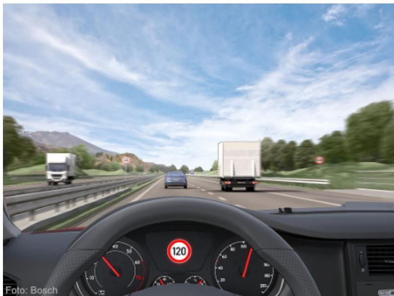
Traffic sign recognition uses a forward-facing video camera mounted in the area of the rear view mirror to permanently monitor road traffic signs.
