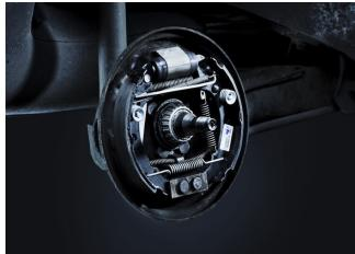
The wheel cylinder is a safety-relevant vehicle part. It should be checked regularly as part of regular service and maintenance to ensure that it is perfect working order. When the brake shoes or the brake drums are replaced, it is advisable to replace the wheel cylinder at the same time. This will avoid follow-up repairs having to be made soon after.
