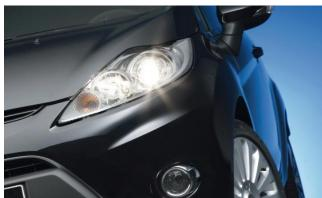
The primary task of headlights on cars is to illuminate the roadway and facilitate fatigue-free and safe driving. Headlights and their light sources are thus vehicle components that are relevant to safety. They require official approval and must not be tampered with. The nature and location of light functions on a vehicle and their design, light sources, colours and photometric values are regulated by law.
