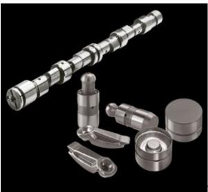
The camshaft is a mechanical component of an internal combustion engine. It opens and closes the inlet and exhaust valves of the engine at the right time, with the exact stroke and in a precisely defined sequence. The camshaft is driven by the crankshaft by way of gearwheels, a toothed belt or a timing chain. With a transmission ratio of 2:1, the rate of rotation of the camshaft is half that of the crankshaft.
