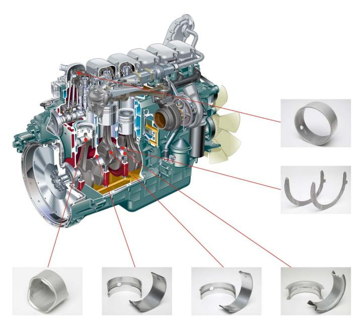
Plain bearings can also be damaged by oil starvation. Oil starvation can be caused by a faulty or leaking oil pump, for example, a fault affecting the pressure limiting valve, a leak in the oil pipe system, too little oil or the vehicle being too sharply tilted.
