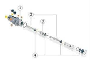
Due to statutory provisions, a car must be equipped with two separate brake circuits. So-called tandem master cylinders generate the hydraulic pressure for the two separate brake circuits. In the event of one brake circuit failing, the brake pressure builds in the other brake circuit still intact.
