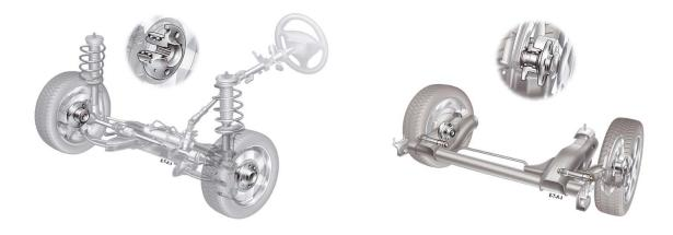
Depending on the design of the bearing, the rolling elements ball or roll-shaped. They roll back and forth on the raceways of the two rings. Their task is to transfer the force acting on the bearing from one bearing ring to the other.
