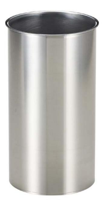
In combination with the piston and the cylinder head, the cylinders of a combustion engine form the working space and combustion chamber. The cylinders are also charged with the task of guiding the pistons as they move up and down and directing the heat generated during the combustion process to the cooling system.
