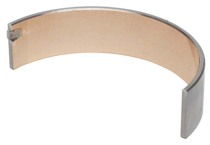
They also have the important task of absorbing and embedding abrasion. This abrasion occurs during normal operation of the engine. It takes the form of tiny particles of metal that are too small to be trapped by the oil filter but big enough to cause increased wear if they are not embedded. This key function of the plain bearing for smooth running and low-wear operation of the engine requires a specific design.
