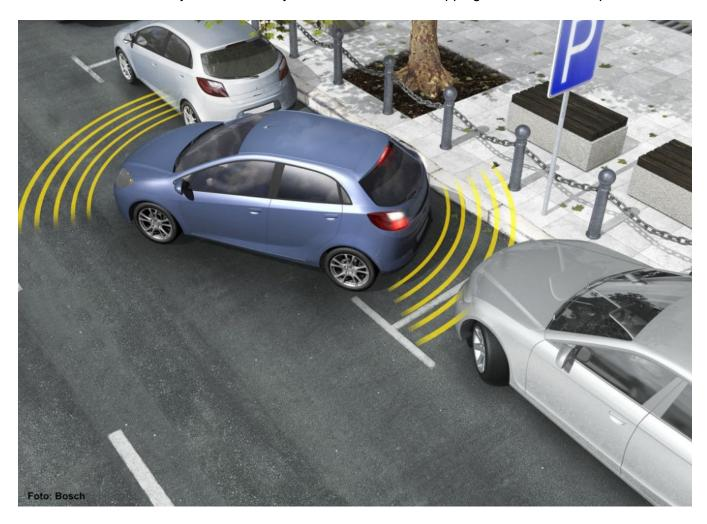
Parking aid systems use ultrasonic sensors integrated into the front and rear end of the vehicle to monitor the area directly in front of and behind the vehicle. To do so, the sensors emit ultrasonic signals and pick up the echo of these. The system determines the distance from the obstacle on the basis of
