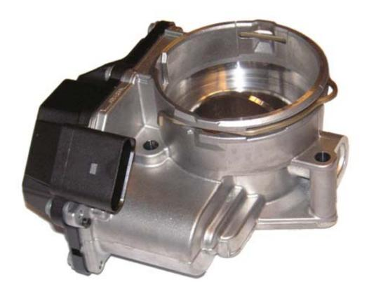
If throttle valves are used in diesel engines, they are generally referred to as air management valves. Air management valves can be with or without integrated control electronics. As indicated above, air management valves throttle the intake air in the intake air system of diesel engines via electromotive means in order to achieve precision controlled exhaust gas recirculation and prevent the inconvenient shaking that would otherwise occur when the engine is switched off.
