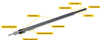
Cross-sectional view of metal rod glow plugs
