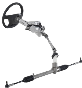
Structure of electric power steering on the steering column ©ZF Aftermarket
