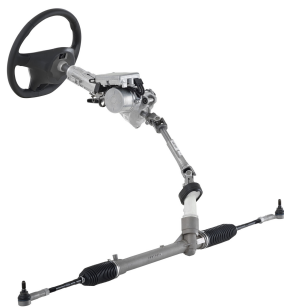
Structure of electric power steering on the steering column ©ZF Aftermarket
